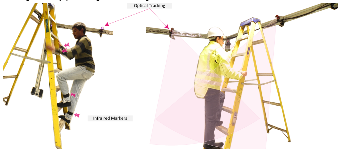
Fig.2 Motion tracking setup for tracking the ladder climbing activity
